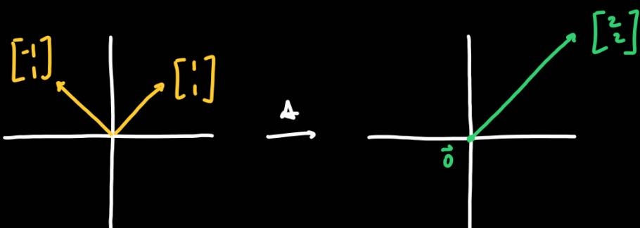
The "preferred directions" are  $\begin{bmatrix} 1 \\ 1 \end{bmatrix}$  and  $\begin{bmatrix} -1 \\ 1 \end{bmatrix}$  with scaling factors of 2 and 0 respectively.
